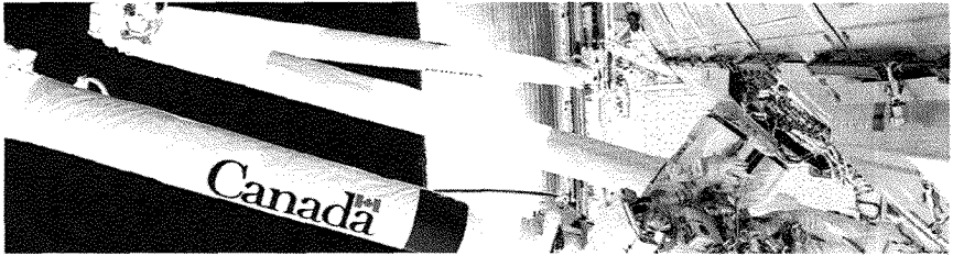
Canada's Space Station Remote Manipulator System can creep slowly along the outside of the space station like an inchworm.
