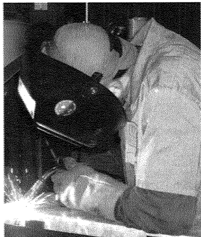
Gas metal arc fillet weld
