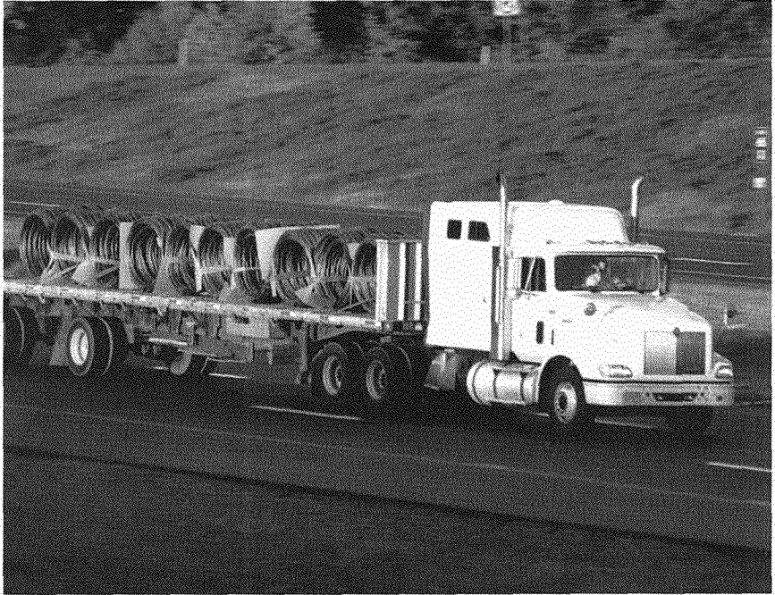
The flatbed truck typically is used to haul very large items that will not fit in a closed truck or that cannot easily be unloaded from the back of a truck trailer.
