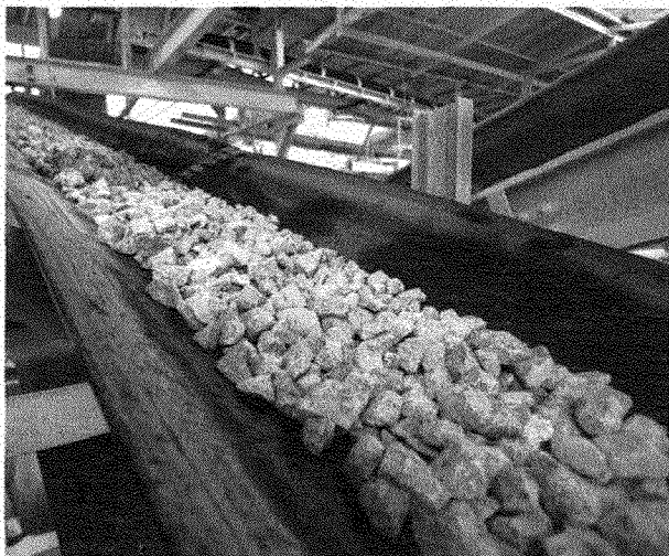
Crushed stone from primary crusher
