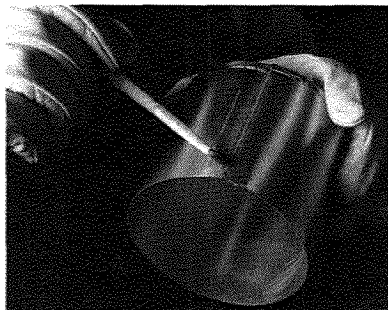
When using an acid flux, wear gloves and goggles, and work in an area with good ventilation.
