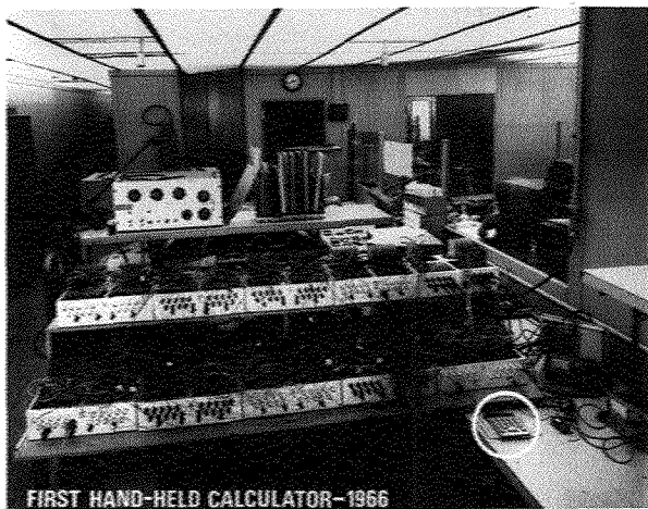
The breadboard (construction base) for the first electronic handheld calculator fills a room.
