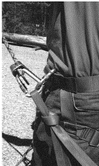
Bottom belay system setup
